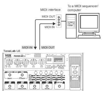
When you connect ToneLab LE with a MIDI sequencer or sound editor, data will normally be sent in both directions, so you will need to connect MIDI cables from ToneLab LE's MIDI OUT jack to the external MIDI device's MIDI IN jack, and from the external MIDI device's MIDI OUT jack to ToneLab LE's MIDI IN jack.
